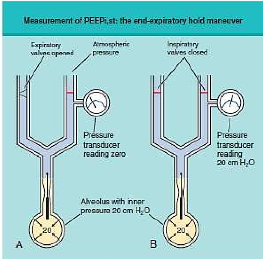
Figure 15.6. Schematic representation of the respiratory system and a ventilatory circuit. A, During the expiratory phase, the ventilator opens the expiratory valve while the inspiratory valve is closed. Consequently, the pressure transducer reads atmospheric pressure. B, At end expiration, both inspiratory and expiratory valves are closed (end-expiratory hold maneuver). The pressure transducer now reads the end-expiratory alveolar pressure.
