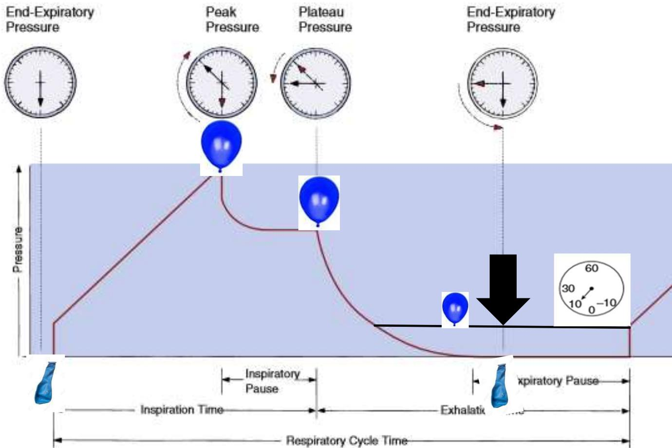
**Figure 3-23** A pressure-time curve for passive positive pressure lung inflation, followed by a momentary inspiratory pause (breath hold) and passive exhalation. Peak pressure and plateau pressure correspond to points B and D in Figure 3-22. (Modified from DuPuis YG: *Ventilators: theory and clinical applications*, ed 2, St Louis, 1992, Mosby.)
